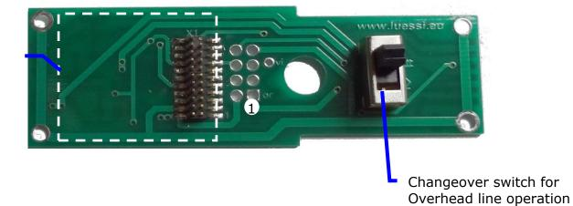
The strands are soldered on at the same place as on the original decoder. (The stranded wire colours in the locomotive are according to Märklin). Contact surface for pantographs
