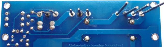
*The two power transistors and the bridge rectifier are first soldered to one leg only.*
