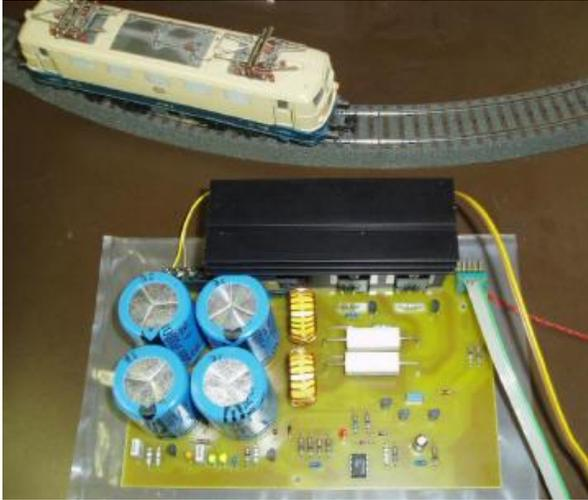
*A simple test setup with a few tracks is sufficient to test the new circuit. A clean workplace is important. (In the picture you can see an older version of the booster.)*
