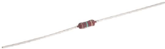
This picture shows a carbon film resistor with 0.3W. This possesses only 4 rings, the first two rings are for the first two digits, the third ring for the number of zeros. The last ring - set off from the other three - indicates the tolerance value ( $\pm 5\%$ ).
