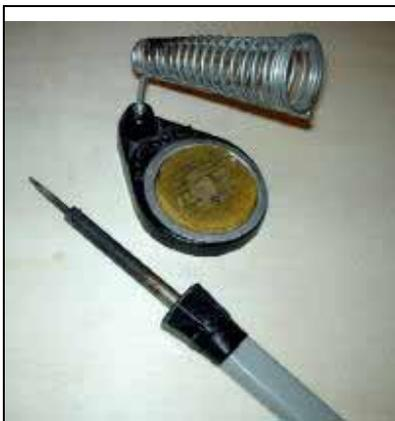
*A cheap soldering iron. This model uses a copper tip which needs to be reshaped every now and again. Professionals have their special form for the point. The filed tip must be tinned immediately.*
