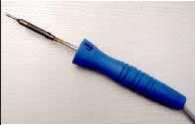
*Here is an other cheap soldering iron. Unfortunately this has a completely useless soldering tip for electronics and model construction work. As you may see in the detailed picture, the tip is not pointed, but simply flattened.*
