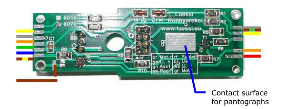
The wires are soldered at the same place as the original decoder. (strand colors in the locomotive are according to Märklin)
